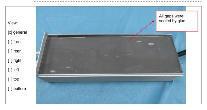
Details of: Internal view for ASN2-RGB (LED driver part)
