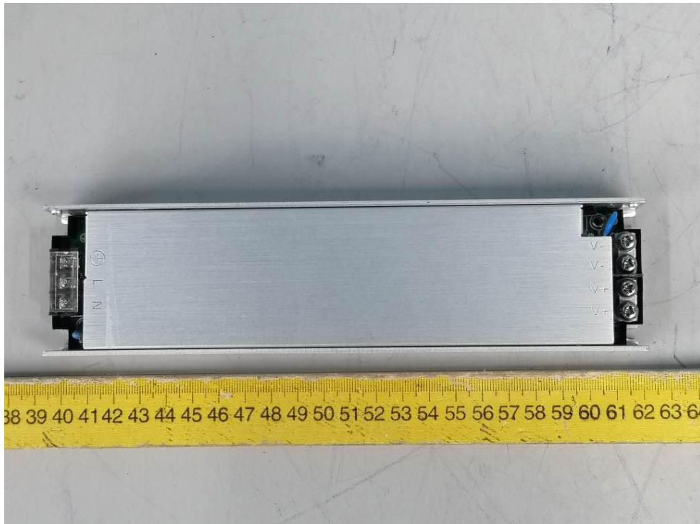
Photo 5 Power supply board view
