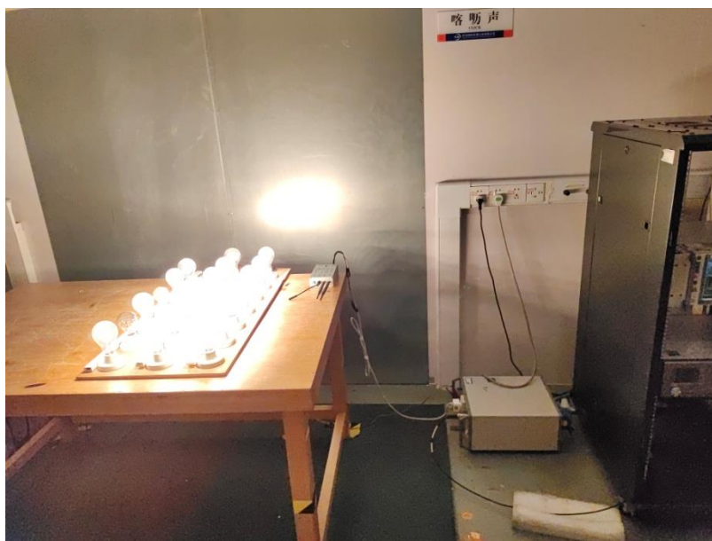
Conducted disturbance at mains terminals Test
