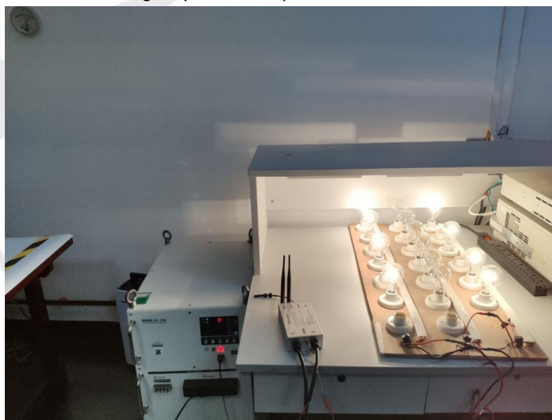
Voltage dips & interruption Test
