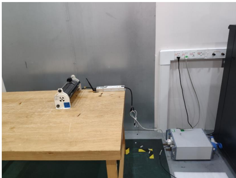
Conducted disturbance at mains terminals Test
