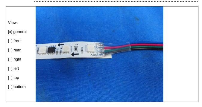
Details of: End terminal view for DN-W-Y-Z-X, same as other models
