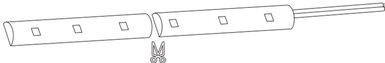
Please cut at the cuttable mark,keep shear level,then power on for test
