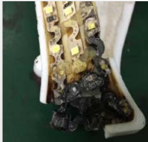
Short circuit caused fire
