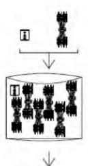
Wrap modules by wire ties and then put into anti-static bag with desiccant
