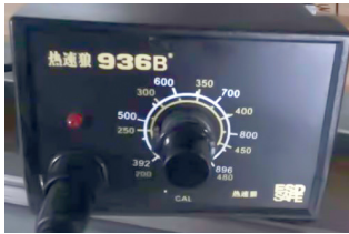
Welding under constant temperature, temperature setting: 250°C ~260°C;
