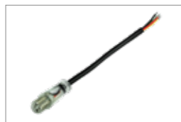
IP64, Clear male connector, 4 cores, UL2464 22AWG L=300/3mm, with 20mm wire
