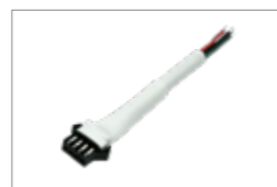
SM-4A male connector, 4 cores, UL2464 20AWG L=70/2.5mm, with 18mm wire
