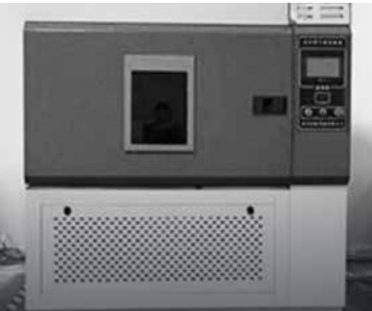
Xenon Lamp Test 336 hours
