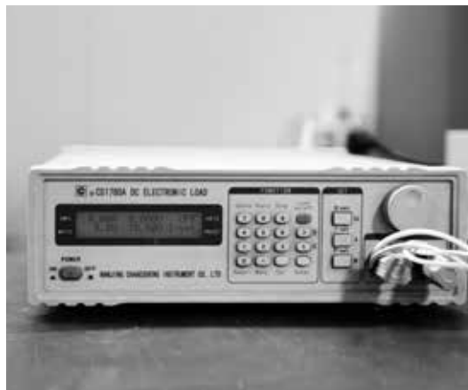
No-load/Load Capacity Test within \pm 0.5V
