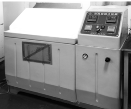
Corrosion Resistance Test 72 hours
