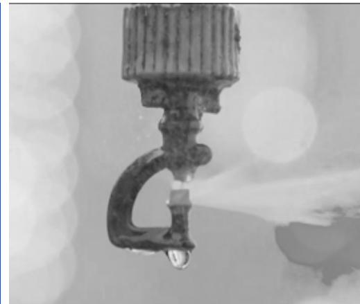
Water spray IPX5/6 standard 336 hours
