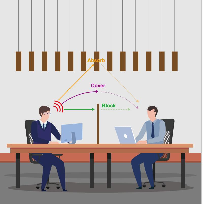
Combining standard-compliant LED workplace lamps with flexible sound insulation panels can best illuminate one or two workplaces while minimizing reverberation and achieving an ideal balance between sound absorption and sound insulation. An optional desk screen separates spaces that require extra privacy. The simple lamp design uses discreet colors to ensure visual tranquility.
