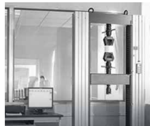
Mechanical Strength IEC60598 4.13
