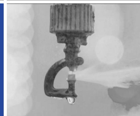
Water spray IPX5/6 standard 336 hours
