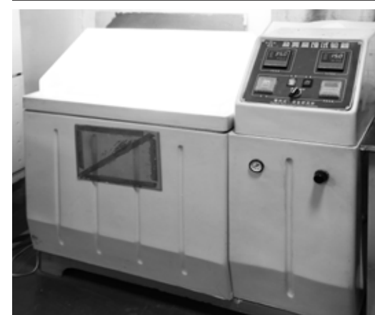
Corrosion Resistance Test 72 hours
